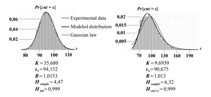
In the two cases the entropy of the raw binary signal exceeds the value 0.997 required by AIS31
